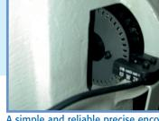
A simple and reliable precise encoding device for mold height and locking force
